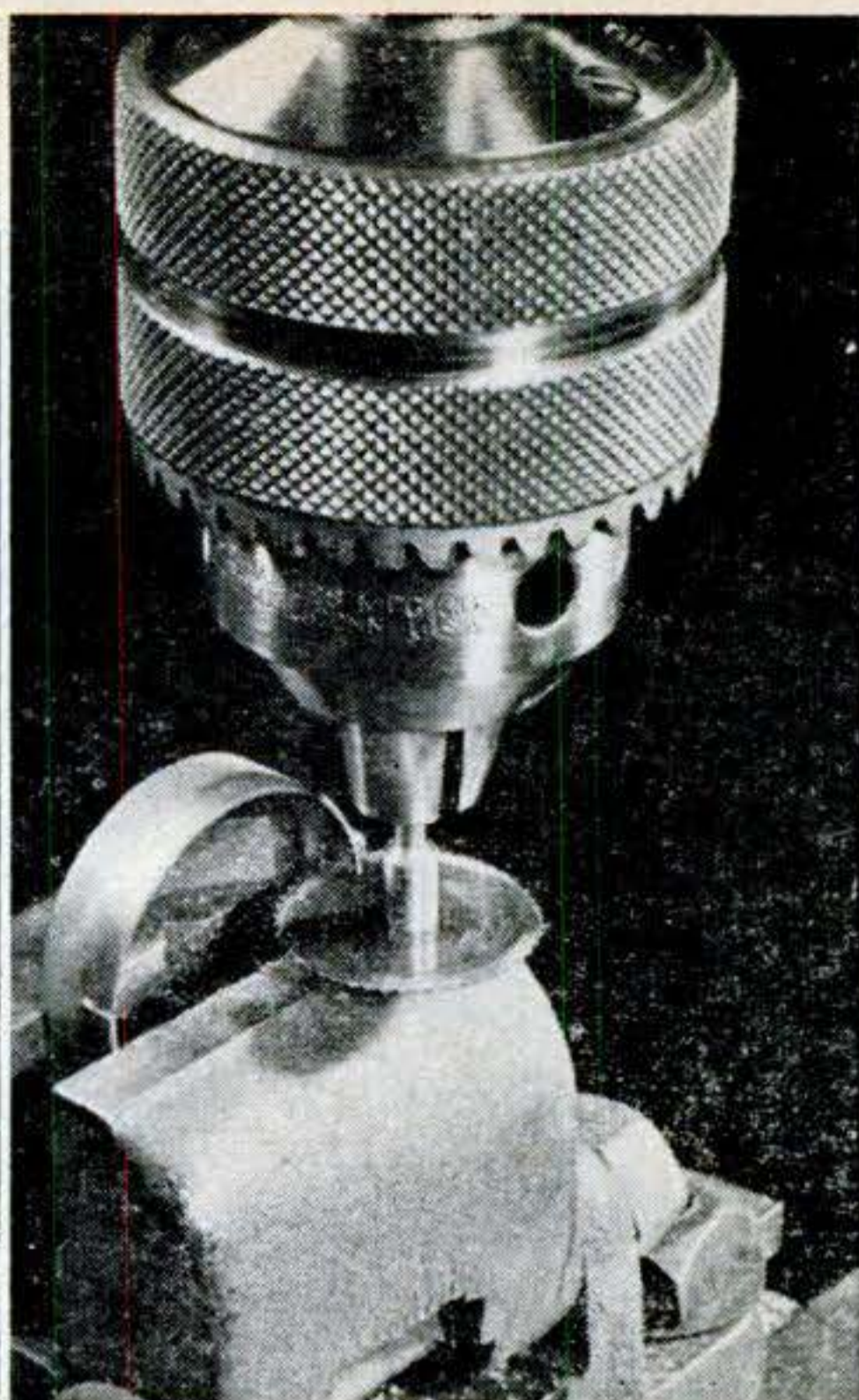
SLITTING SAW mounted on arbor is useful for making split rings and bushings or slotting screwheads. Slits in collet chucks are easily cut.
